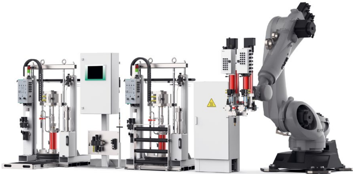
Hot butyl dual dosing system for seals with processing temperatures of up to 180 °C
